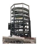
This compact machine, fitted with the proven and patented Triple-E spiral conveyor belt, offers much smoother transportation and needs less maintenance. With up to 110 metres of accumulation length and speeds of up to 35,000 units per hour, it is the clear market leader.
